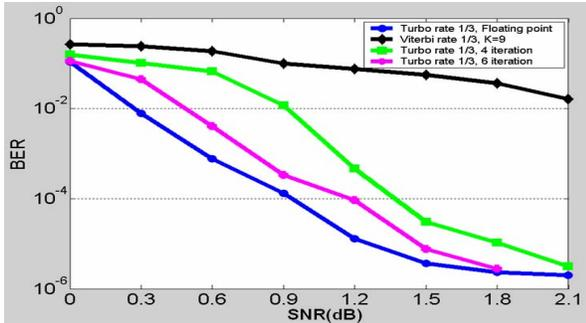
Figure 6. Finite precision performance of triple-mode MAP/VA IP
