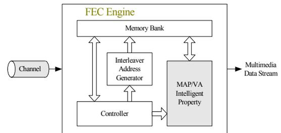
Figure 1. The proposed unified FEC engine.
