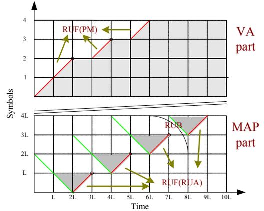
Figure 3. Timing chart of triple-mode decoding (Convolutional codes with  $K=9$  and Turbo codes with  $K=4$ ).
