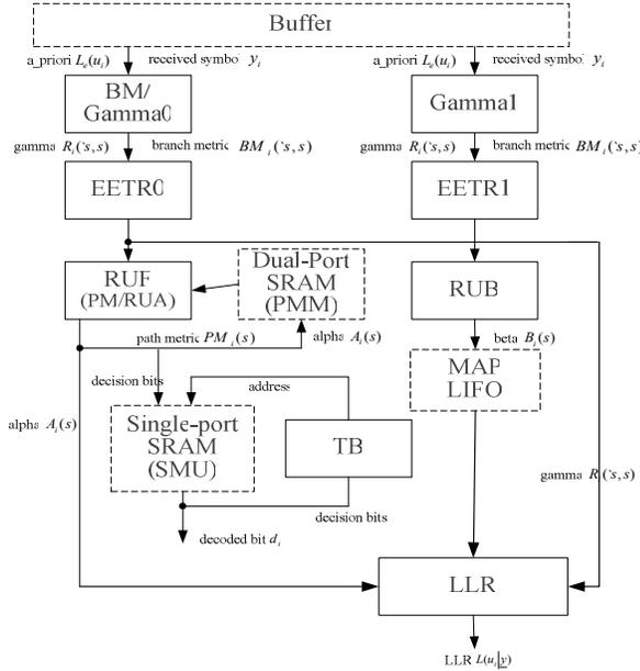
Figure 5. Architecture of the triple-mode MAP/VA IP
