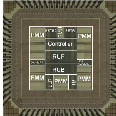
Figure 7. Die photo of the triple-mode MAP/VA IP.
